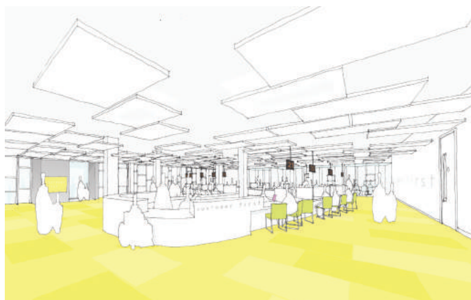
May 2005. Sketch of One Stop Shop showing 'sock desk', rubber floor finish and the ceiling system composed of Barrisol light panels, aluminium radiant panels and acoustic panels
